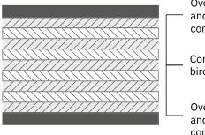
Overlay: wood fibre and polypropylene composite
