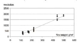
The Small Mesh wear resistance to wear parameters are superior to those of the Large Mesh. By using special overlays it is possible to produce plywood with a wear resistance to even above 10 000 revolutions.
